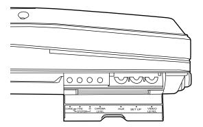
The video signals (ENCODER OUT) must be adjusted upon completion of the system connections before any signals are transmitted in order to conduct accurate error-free editing.
