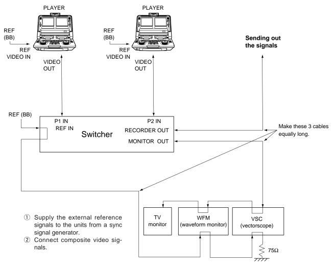
If a waveform monitor and vectorscope are unavailable, observe the images on a monitor and adjust to eliminate any color shifting.
