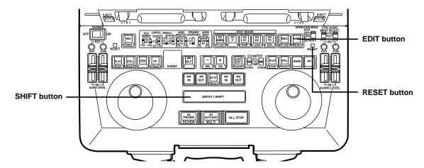
To transfer the laptop from the regular mode to the set-up menu mode, press the SHIFT and EDIT buttons together. (This cannot be done by remote control, or when editing or recording.)
