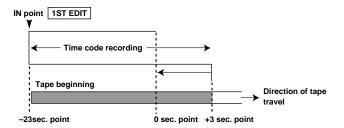
For insert editing, the control signal must be recorded from the start to the end of the editing tape.
