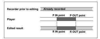
• If it is necessary to maintain the continuity of the time codes on the tape in the recorder during TC insertion, set set-up menu item No. 507 (TC MODE) to "I-REG". When the setup menu No.507 is set to "P-REC" or "P-FREE", set set-up menu item No. 510 (REGEN MODE) to "AS&IN" or "INSRT."
