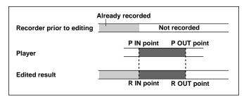
• In order to maintain the continuity of the time codes on the tape in the recorder, set set-up menu item No. 507 (TC MODE) to "I-REG". When the setup menu No.507 is set to "P-REC" or "P-FREE", set set-up menu item No. 510 (REGEN MODE) to "AS&IN" or "ASSEM."
