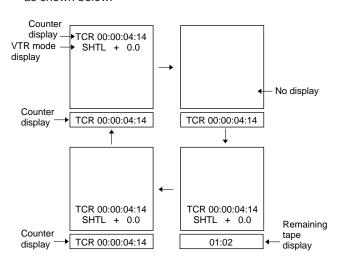
\* The display shown above appears on the LCD monitor only when set-up item No.001 (LCD SUPER) is set to ON.
